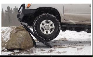
PROVIDES TRACTION/CLEARS DEBRIS
